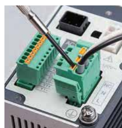
The power and I/O connectors are of the screwless type.
